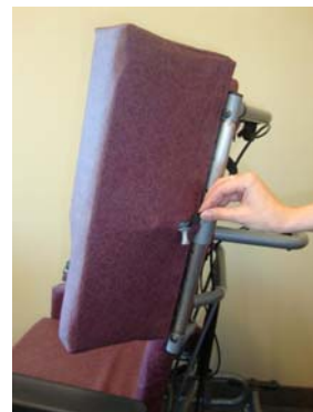
Once wing is locked into place, tighten wing nut.
